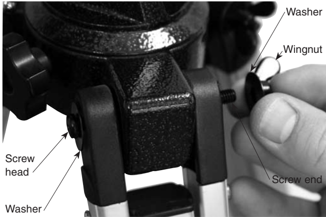
Figure 2. Attach the tripod legs to the mount with the screws that come installed in the tops of the tripod legs. One washer should go between the screw head and tripod leg and the other washer should go between the wingnut and tripod leg.
