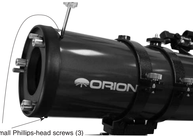
Figure 15. To remove the mirror cell from the telescope, the three small Phillips-head screws on the perimeter of the mirror cell must be completely unthreaded.
