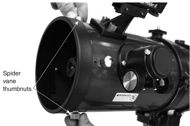
Figure 11. To center the secondary mirror up-and-down in the focuser drawtube, make adjustments to the two knurled spider vane thumbnuts that are perpendicular to the focuser.
