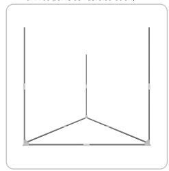
O4. Complete another triangle frame on the three vertical bars using connectors to complete the stand as shown below.
